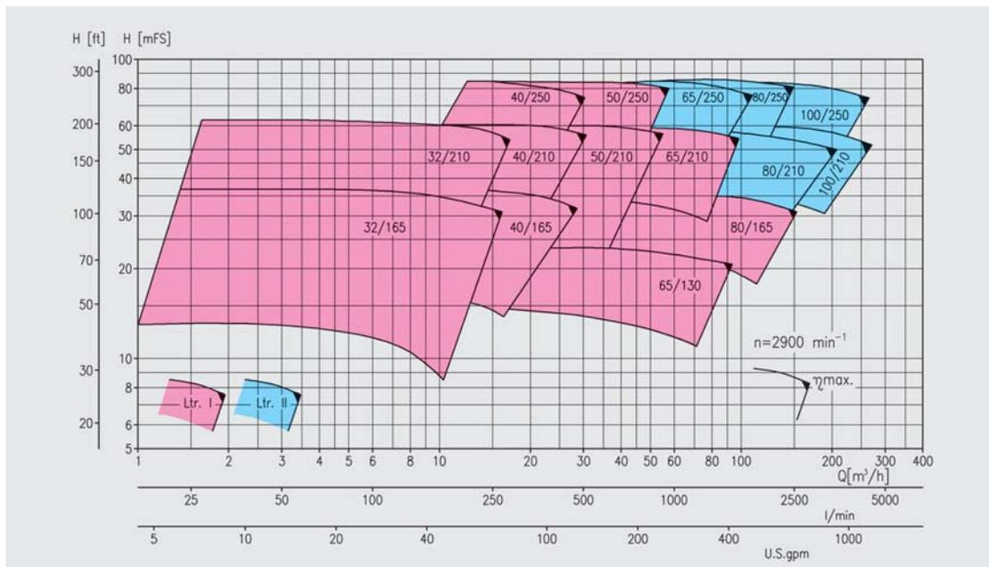
Performance curves of the individual pump sizes, also for 1750 / 3500 rpm, are available on request.
