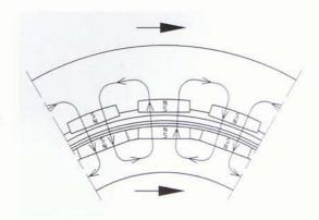
The inner magnet ring transmits the required torque direct to the impeller. Overload of the magnetic coupling and slipping will not affect demagnetization if a reliable monitoring device prevents overheating of the magnets.
