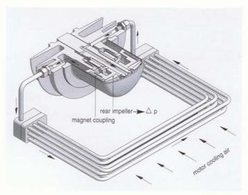
For a drive power higher than 22 kW and magnetic losses above 2,0 kW, an additional external cooling loop is required. The rear impeller on the rotor creates a circulation which cools down the heated liquid (by the containment shell) trough the external cooler by dissipation to the atmosphere.
