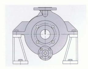
Centerline mounted design is available on request. Capacity and flange to flange dimensions comply with DIN EN 22858.
