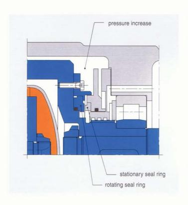
The slide rings of the secondary seal operate without contact and wear free. The seal will be activated only if the containment shell leakage leads to a pressure increase in the bearing bracket.
