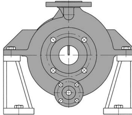
The casing forms - together with the containment shell - the pressure retaining pump part. Maximum allowable pressure at PT is determined by the shell design and the material. The pump casing has metal-to-metal fits with confined compression controlled gaskets.
