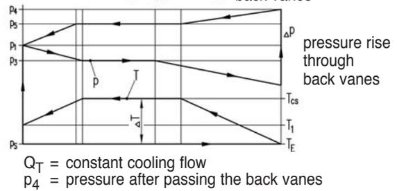
The cooling flow is led from the discharge side behind the impeller into the chamber between the slide bearings and through the pump shaft via the rotor back vanes again to the discharge side. This design pressurizes the slide bearings and the containment shell with nearly the full discharge pressure and the product remains stable in this area.
