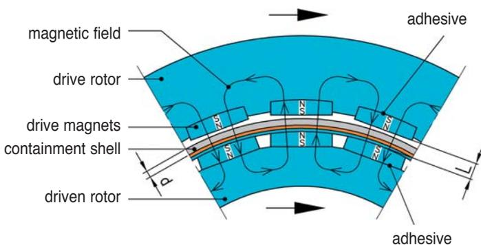
The magnetic couplings are designed to transmit rated motor power up to 220 kW (295 hp) at 2900 rpm, respectively 260 kW (348 hp) at 3500 rpm. The couplings are sized to fit the maximum power consumption of the rated impeller and allow also at least 5% increase of the installed impeller diameter. If nothing else is specified, the transmissible coupling power, the rated motor power and the available moments of inertia are sized for direct-on-line starting of the electric motor.
