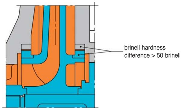
Mating wear surface materials have a difference in Brinell hardness of at least 50 HB.
