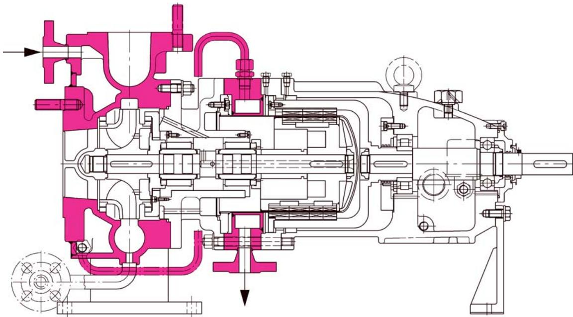
For handling fluids with melting temperature above ambient. Design data for heating jacket 24 bar / 250°C (485°F).
