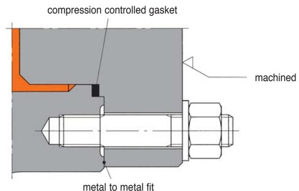
Pump flanges are full or spot faced on the back and designed for through-bolting.
