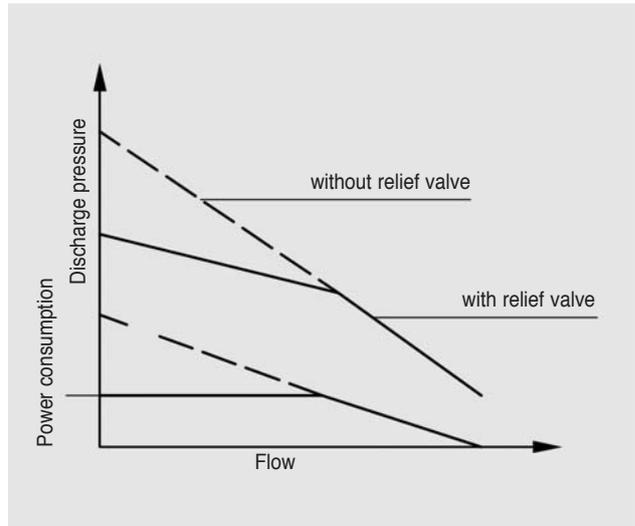
Contrary to centrifugal pumps, the side channel pumps generate a steep head rise and an increased power consumption at lower flow rates. Power consumption and discharge pressure reach the maximum at closed discharge valve. To protect discharge pipes and to avoid overload of the motors, additional relief valves can be fitted to the WPC-pumps.
