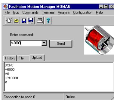
All motor parameters for pump control can be set and saved with »Motion Manager« operating under Windows®. The program language is ASCII-based. Dosage programs can easily be typed on a computer and transferred to the EEPROM.
