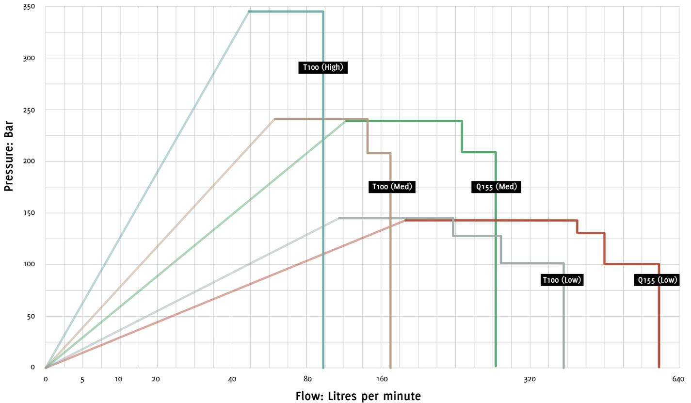
The graph above displays the maximum flow capacity at a given pressure for each model series. The table below lists the maximum flow capacity and maximum pressure capability of each model series.
