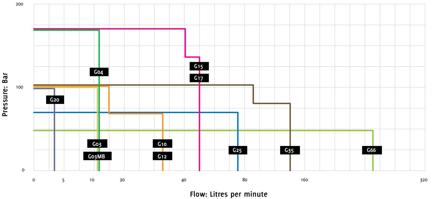
The graph above displays the maximum flow capacity at a given pressure for each model series. The table below lists the maximum flow capacity and maximum pressure capability of each model series.
