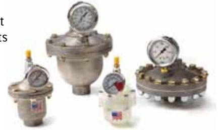
They control pulsations by allowing fluid to enter a wetted chamber of the dampener during the discharge stroke. This displaces a flexible bladder, which compresses gas in an air chamber, thus absorbing the shock. During the inlet stroke, liquid pressure decreases as the dampener gas expands, allowing fluid to re-enter the process line.
