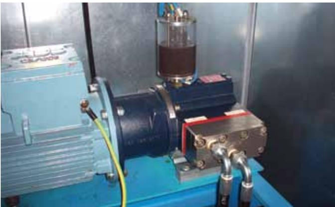
*High-precision dosing of pentane at low flow rates can be achieved for specialised applications in polyurethane processing.*
