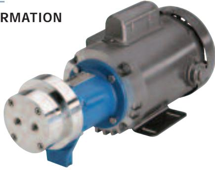
Liquiflo's **4-Series** pumps are low-flow magnetically-driven external gear pumps that are completely field repairable. The 4-Series housings are manufactured from Bar Stock in 316 Stainless Steel, Alloy-C or Titanium. With several material options for shafts, gears, wear plates and bearings, these pumps can be used in a wide variety of chemical processing applications.
