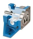
Gerotor pumps are <u>internal gear pumps</u> without the crescent. The rotor is the internal (drive) gear shown below in gray, and the idler is the external (driven) gear, shown below in orange. They are primarily suitable for clean, low pressure applications such as lubrication systems or hot oil filtration systems, but can also be found in low to moderate pressure hydraulic applications.
