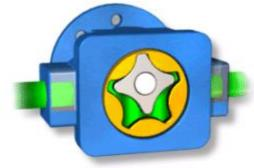
Rotor and idler teeth mesh completely to form a seal equidistant from the discharge and suction ports. This seal forces the liquid out of the discharge port.
